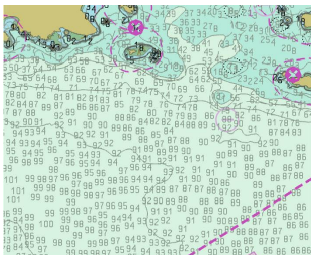
Figure 2. Example of the hydrographic sounding selection from a high-resolution survey.
