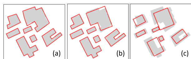
Figure 2. Three different building simplification algorithms available in CartAGen: (a) building simplification from the AGENT project (Barrault et al., 2001), (b) recursive regression (Bayer, 2010), (c) simplify to rectangle (Barrault et al., 2001).
