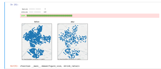
Figure 12. Extract of a CartAGen notebook showing the results of a point selection algorithm based on a K-means clustering with two slide bars that help adjusting interactively the parameters of the algorithm.
