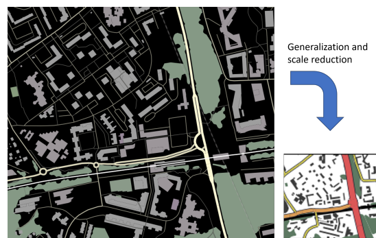
Figure 13. Topographic data generalized in many steps with the topographic generalization notebook of CartAGen.
