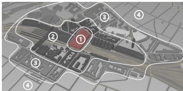
Figure 2: Schematic visualisation of four generalisation levels: (1) detailed building in focus, highlighted in red; (2) detailed buildings in dark grey; (3) generalised buildings in grey; (4) generalised block edges in light grey.
